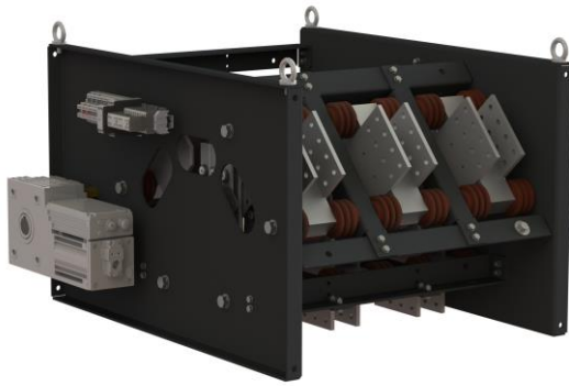
MVI-CI30Y 3.6kVac 7200A 3p with 3 positions and central neutral position with motor M 3x400Vac with control 1x230 Vac by Siemens PLC
